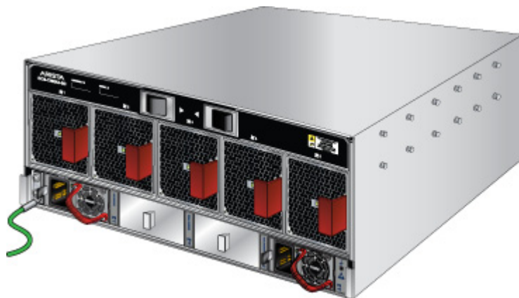
Figure 4-1: Grounding Pad and ESD Grounding Pad Sockets
